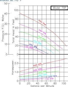
The liquid flow varies directly as the pump speed-the higher the speed the greater the flow. Horsepower required varies directly as flow and pressure. Maximum horsepower is required with a wide open discharge line. This is the point of maximum flow. With a throttled discharge, the flow decreases at a greater rate than the pressure increases thereby requiring less horsepower at the higher pressures. This is known as an "unloading" feature of the pump.
